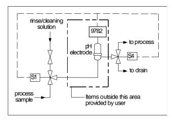
Figure 15-11 Automatic Electrode Wash Setup
